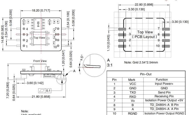
Unit: mm[inch] Pin diameter tolerances:  $\pm 0.10[\pm 0.004]$ General tolerances:  $\pm 1.0[\pm 0.039]$
