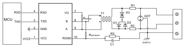
Fig. 2: Port protection circuit for harsh environments
